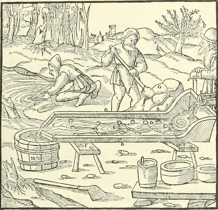
A—HEAD OF THE SLUICE. B—SIDE-BOARDS. C—LOWER END OF THE SLUICE. D—POCKETS. E—GROOVES. F—STOOLS. G—SHOVEL. H—TUB SET BELOW. I—LAUNDER.
